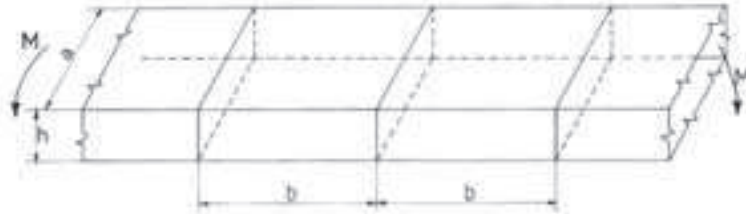
Figure 1: Constant section two spar wing box with equidistant ribs.
